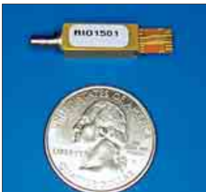
Figure 1. Small form factor TOSA based on PLANEX technology.
